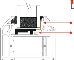
SECURI-CLIP Use SC104 for 28mm units Use SB000 Base Plate with GT002 Black Packer
